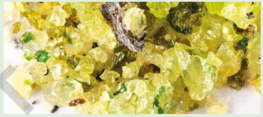
FIGURE 3 Olivine crystals show two different colours depending on whether they are oxidised or not. Orange crystals are oxidised and green are not.
