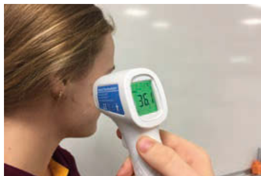
FIGURE 5 An infrared pyrometer allows you to measure temperature without making physical contact. Normal skin temperature varies between 33^{\circ}\text{C} and 37^{\circ}\text{C} .
