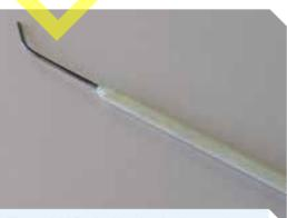
Figure 1.14 Probe Used to look at and explore a specimen, and to probe openings.
